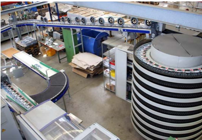
▲ Cooling tower of the perfect binder line installed with Weiss-Druck in Monschau.
